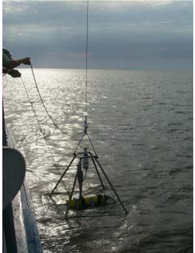
Acoustic instrumentation designed to measure boundary layer turbulence and vertical profiles of current and Reynold's stresses deployed off the Georgia coast.
